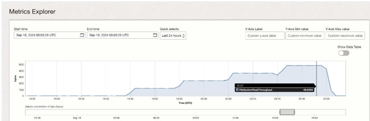
Figure 8. Scaling Out Mount Targets from 1 to 4—Throughput to File System Reaching 48 GB/s
